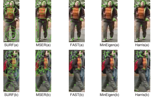
Fig. 3. Key points extracted by different detectors. The first row is from camera A, and the second is from camera B.
